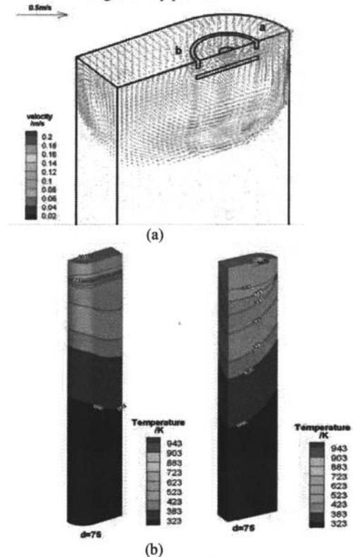
Fig. 4 Velocity vectors (a) and temperature profile (b) during EMA-DC casting process
