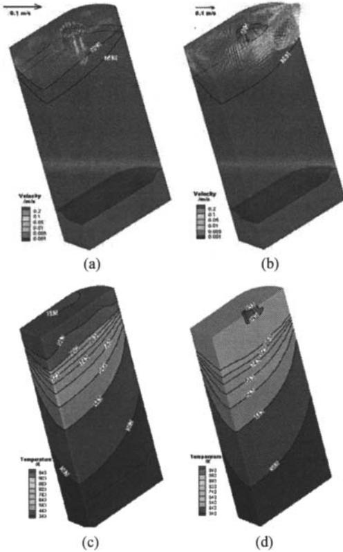
Fig. 2 Velocity vectors and temperature profile during DC casting (a)(c) and EM-DC casting (b)(d) process.
