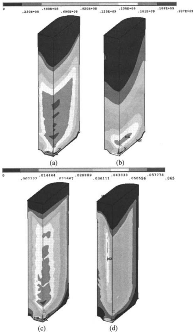
Fig. 6 Equivalent plastic stress and strain profile in the ingots in EM-DC casting (a)(c) and EMA-DC casting (b)(d) processes.
