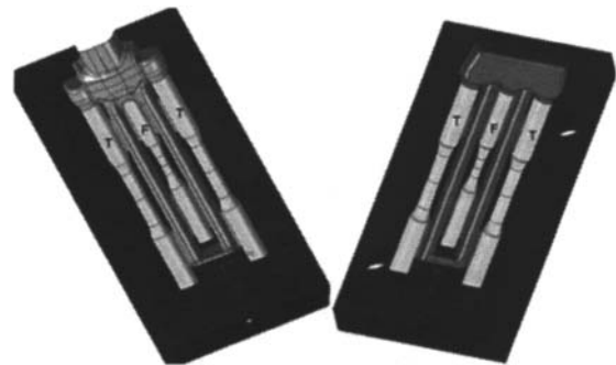
Figure 8. Die Mold cavity for the tilt pour gravity casting of tensile test bars [23].
