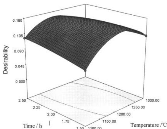
Fig. 8 Effect of calcination temperature and holding time on the comprehensive performance of  $\alpha$ -alumina
