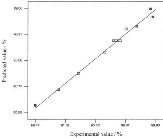
Fig. 4 Comparison of model prediction with the experimental data for yield of  $\alpha$ -alumina
