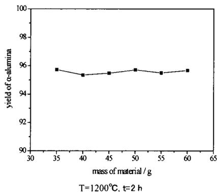
Fig. 3 Effect of the mass of material on yield of  $\alpha$ -alumina
