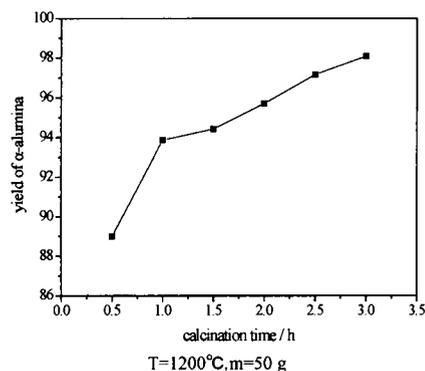
Fig. 2 Effect of the calcination time on yield of  $\alpha$ -alumina
