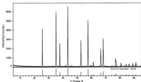
Fig. 9 The XRD pattern for the decomposition final solid products under the optimization conditions
