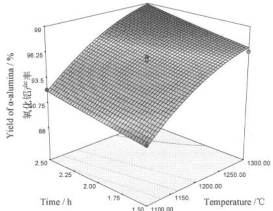
Fig. 6 Effect of calcination temperature and holding time on the yield of  $\alpha$ -alumina
