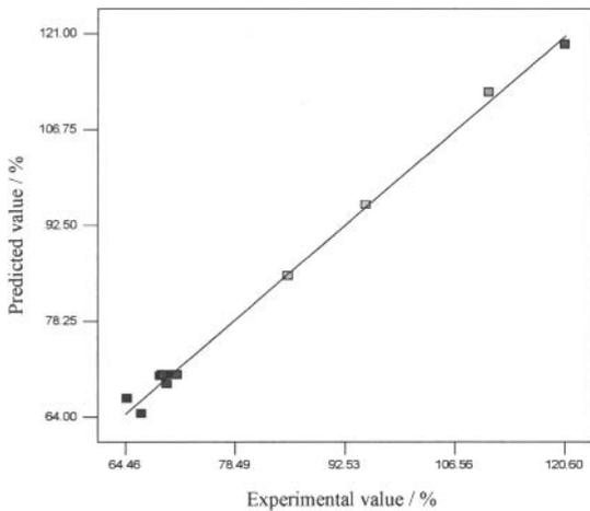
Fig. 5 Comparison of model prediction with the experimental data for average crystal size of  $\alpha$ -alumina
