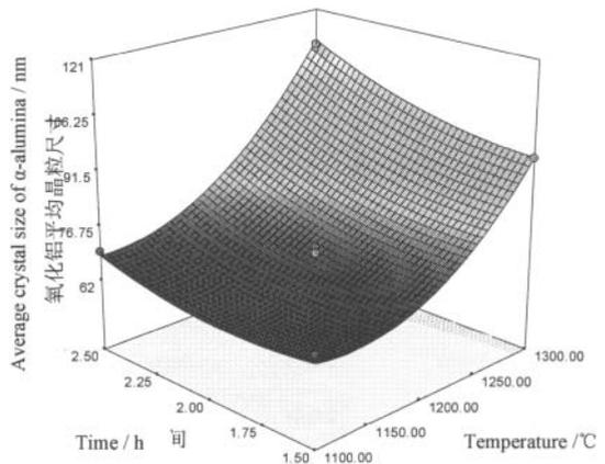
Fig. 7 Effect of calcination temperature and holding time on the average crystal size of  $\alpha$ -alumina
