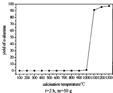
Fig. 1 Effect of the calcination temperature on yield of  $\alpha$ -alumina
