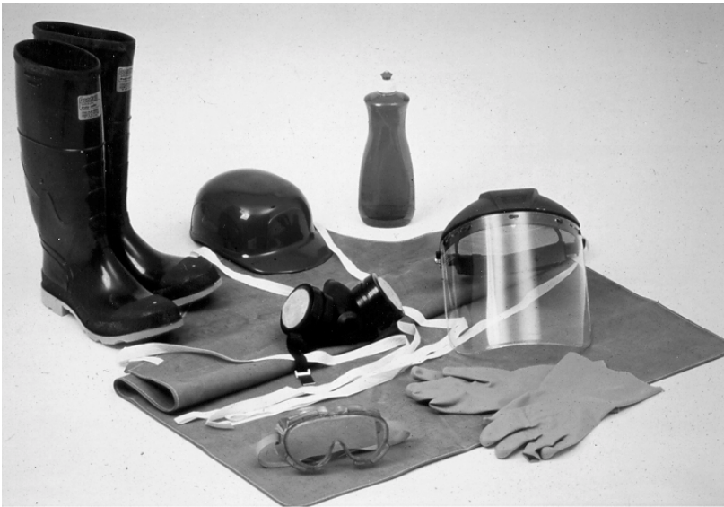
Figure 6.11 Assorted PPE including chemical goggles and face shield (courtesy of University of Wisconsin-Extension).
