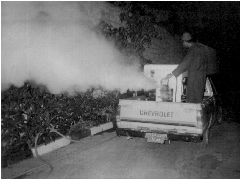
Figure 8.18 Fogger mounted on a vehicle.
