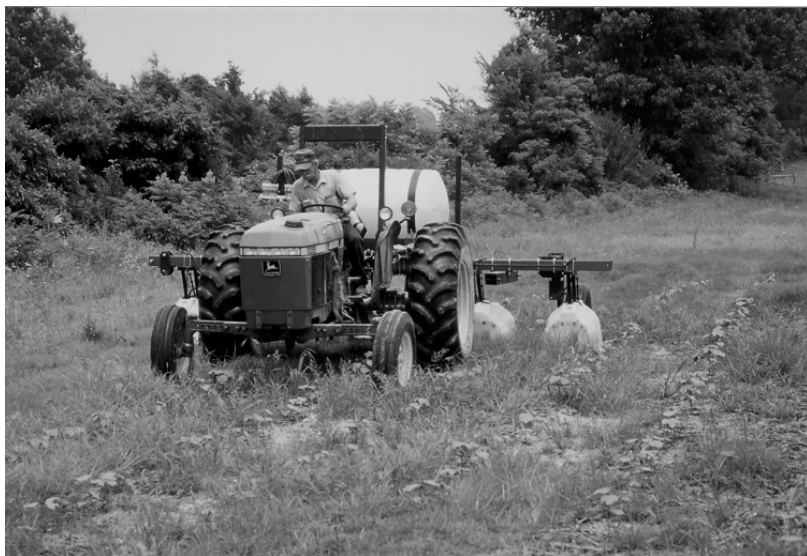
Figure 6.6 Application of a contact herbicide by vehicle (courtesy of Monsanto).
