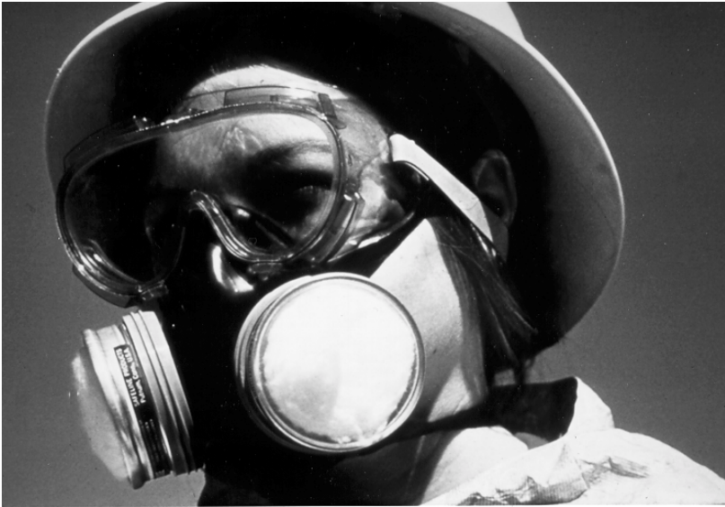
Figure 6.14 Air-purifying respirator-half mask. Worker is also wearing goggles with indirect air vents and a large brimmed hat for protection (courtesy of University of Wisconsin-Extension).
