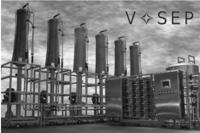
Figure 3.4 Industrial VSEP vibrating modules (Courtesy of New Logic Research).
