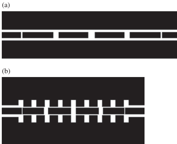
FIGURE 2.30 Layouts of the conventional (a) and periodic-loaded (b) CPW bandpass filters. The layouts are drawn to scale, the length of the conventional filter being 5.6 cm. Reprinted with permission from Ref. [54], copyright 2004 John Wiley & Sons.
