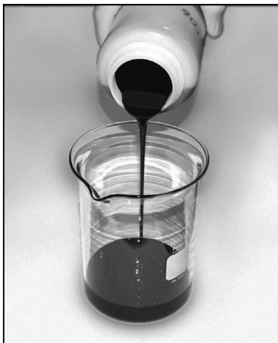
FIG. 8.6 Bio-oil from the fast pyrolysis of lignocellulosic biomass.
