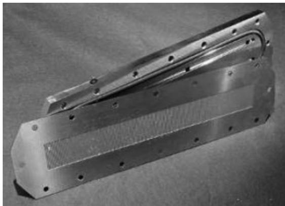
**Figure 10.1** Internal view of the IMVT laboratory-scale microreactor used for experimental determination of optimal reaction conditions and residence time.
