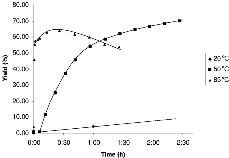
**Figure 10.2** Representative kinetic data for the reaction applied, showing that higher reaction temperature reduces substantially the reaction time required.
