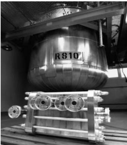
**Figure 10.3** The microreactor before the conventionally used  $10\text{-m}^3$  stirred vessel in the plant, just prior to installation.
