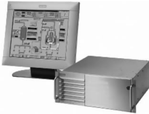
Figure 8.6 SIMATIC PCS7 operator station with basic hardware.
