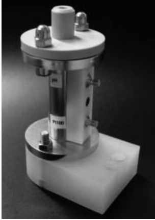
Figure 8.12 pH sensor from JUMO ( www.jumo.net ) with flanges 1/4 in UNF thread.
