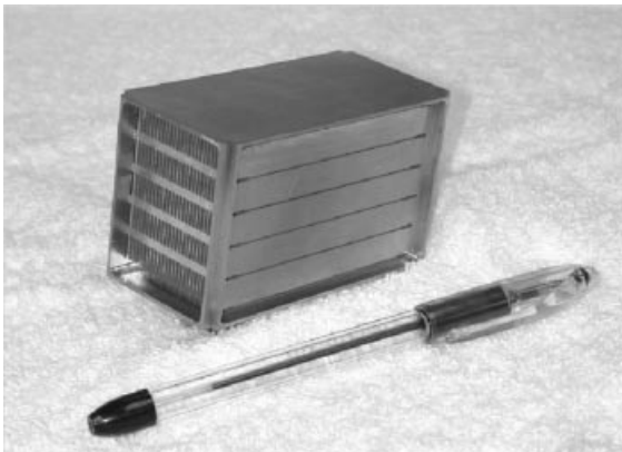
Figure 26.5 2 kW WGS microreactor with incorporated heat exchanger [27].
