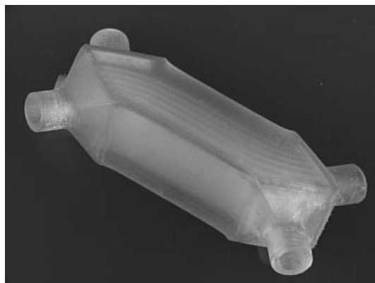
Figure 2.18 Counterflow design microstructured heat exchanger made by microstereolithography.
