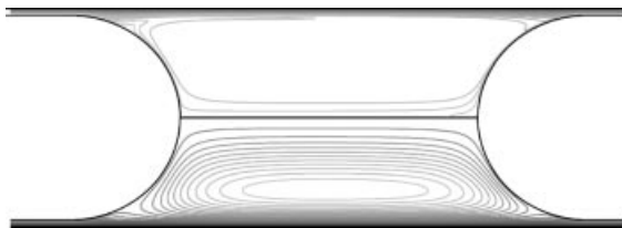
Figure 11.6 Mass transfer in segmented gas–liquid flow. Concentration contours for 20 equally spaced intervals between 0 and C^* are shown in the top half and streamlines are shown in the bottom half for a simulation with D = 1.4 \times 10^{-8} \text{ m}^2 \text{ s}^{-1} , U = 0.4 \text{ m s}^{-1} , d = 1.0 \text{ mm} , L_S + L_B = 4d_h and liquid volume fraction \epsilon = 0.5 [44].
