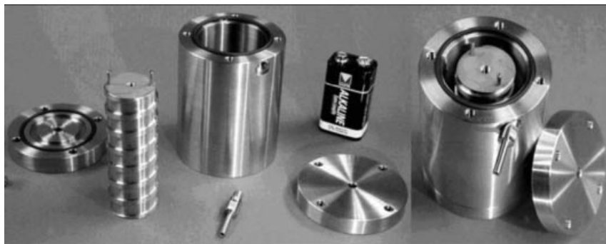
Figure 8.15 Disassembled and partially assembled helicoidal microchannel falling film contactor with path length 540 mm. From [97].
