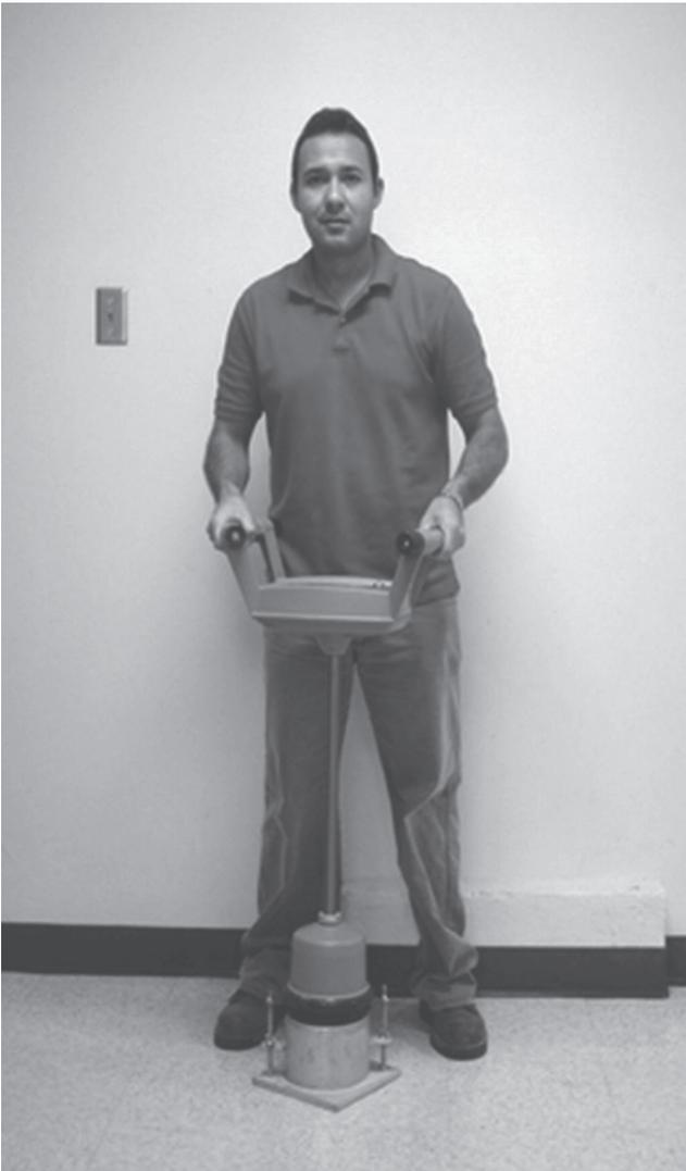
Figure 20.6 BCD-Proctor laboratory compaction test for modulus determination.
