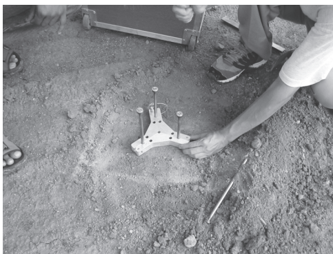
Figure 8.20 Example of time domain reflectometry field probe. (Courtesy of Professor Vincent Drnevich, Purdue University)
