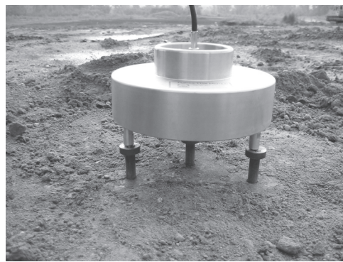
Figure 8.20 Example of time domain reflectometry field probe. (Courtesy of Professor Vincent Drnevich, Purdue University)
