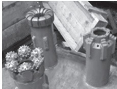
Figure 6.21 Bottom of drill pipes with drill bit. (Left: Courtesy of Rok Max Drilling Tools, Ltd.; Right: After Richards and Zuidberg 1985.)
