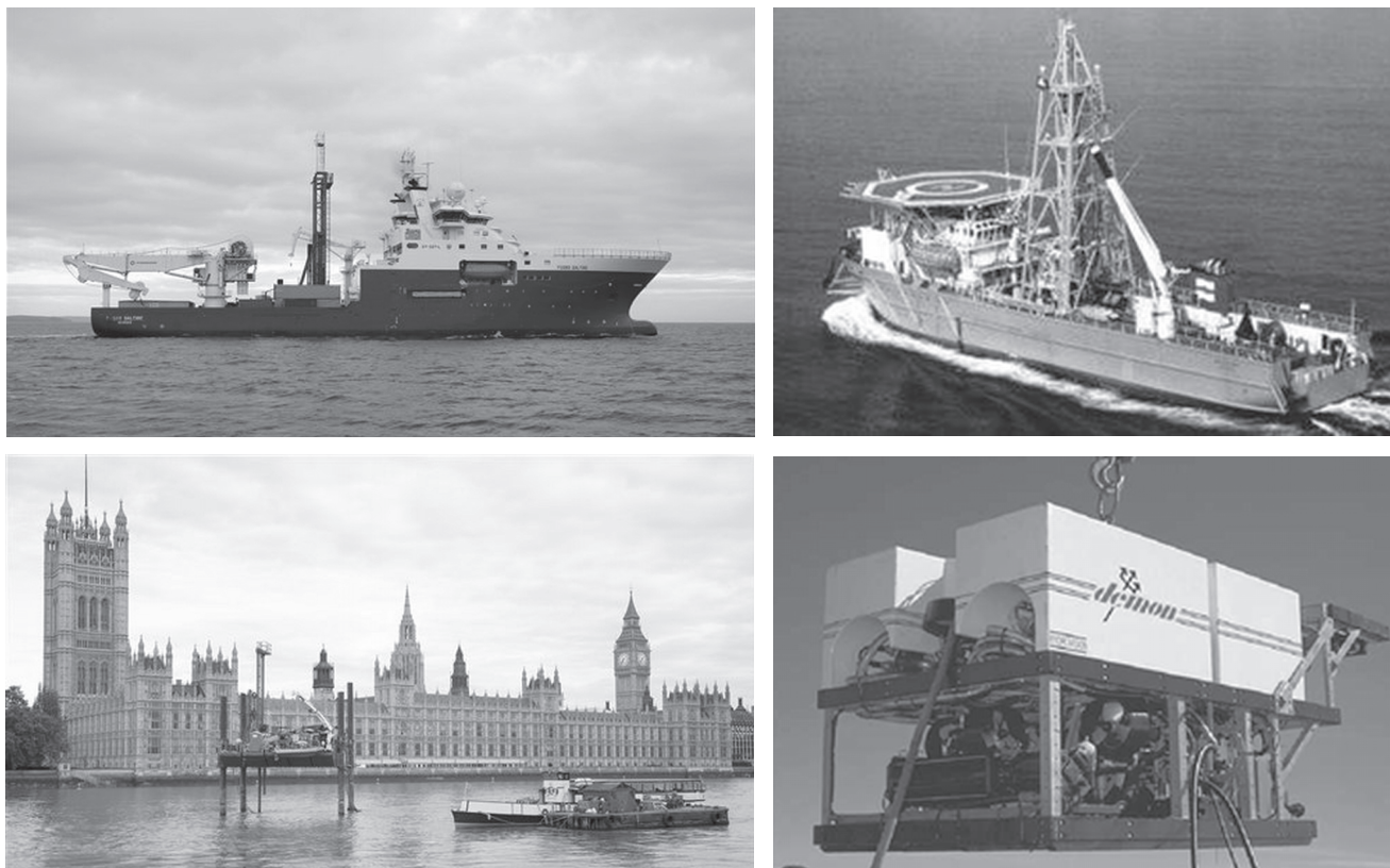
Figure 6.17 Ships, jack-up rig, and remotely operated vehicle (ROV) for offshore investigations. (a, and c: Courtesy of FUGROSeacore., b and d: Courtesy of the ISSMGE Technical Committee on Offshore Geotechnics)
