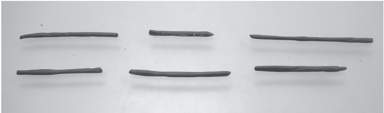
Figure 4.10 Plastic limit test and soil threads.
