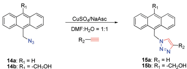
Scheme 14.7 Fluorogenic reaction of azido-anthracene 14 . Reprinted with permission from F. Xie et al., (2008), A fluorogenic “click” reaction of azidoanthracene derivatives, Tetrahedron , 64 (13), 2906–2914. Copyright 2008 Elsevier.
