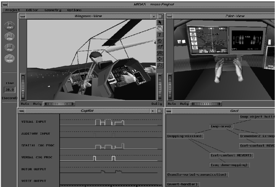
Figure 22 Illustration of a Run-Time View of the MIDAS System with Cockpit, Pilot, and Copilot, and an Activity and Load Time as Well as the Procedures and Goals That Are Currently Active in the System.
