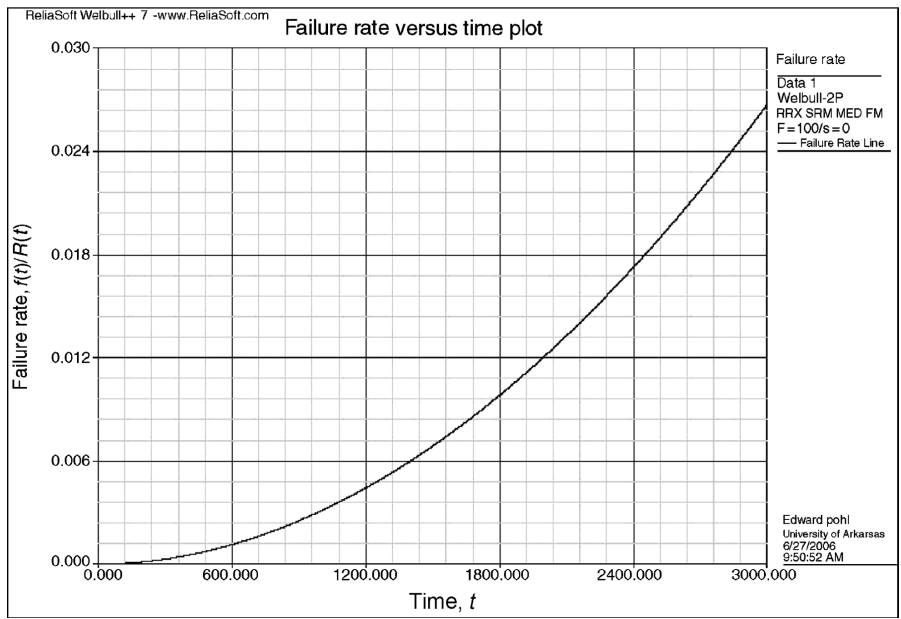
Figure 8.8 Weibull PDF and hazard function, \beta = 2.96 .
