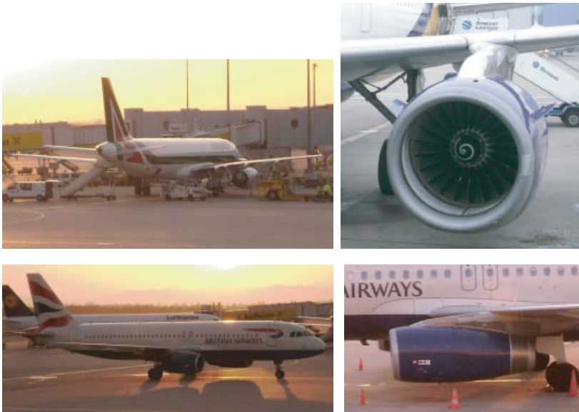
Figure 2.1 Airbus 320 can be fitted with either Rolls-Royce or General Electric jet engines. Spot the different cowlings.
