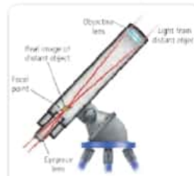
Figure 17 A refracting telescope uses an objective lens and an eyepiece lens to gather light from distant objects so that scientists can observe and study those objects.
