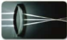
Figure 9 A convex lens bends light inward, toward the optical axis. A light ray that passes straight through the center of the lens does not refract. Identify the focal point of the lens.
