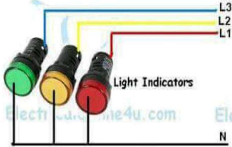
Led Indicator Wiring Diagram for 3 Phase 4 Wire System
