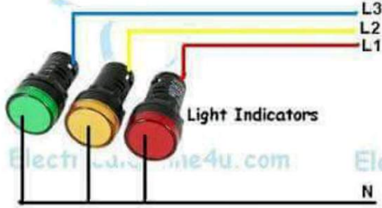
Led Indicator Wiring Diagram for 3 Phase 4 Wire System
