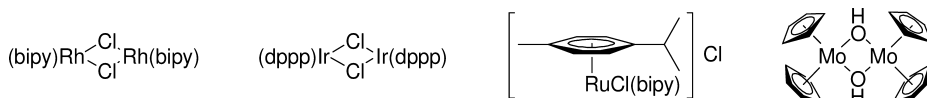
Fig. 20.1 Examples of catalysts operating via the same mechanism as the Wilkinson catalyst (bipy=bipyridine; dppp=1,3-bis(diphenylphosphinopropane) [35, 44, 45].
