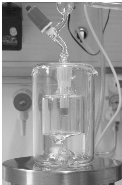
Fig. 10.7 An apparatus used to monitor hydrogenations at different hydrogen partial pressures.
