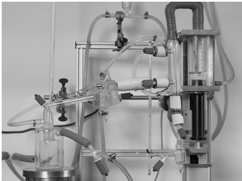
Fig. 10.3 Normal pressure hydrogenation device for the automatic registration of hydrogen consumption under isobaric conditions.
