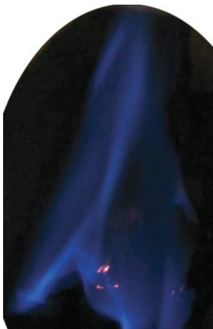
Figure 38.2 Near-stoichiometric flame from natural gas fire. The red glow is from a lava rock bed.
