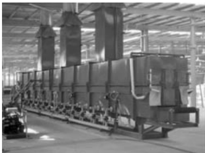
Figure 31.6 ICE wire line equipment fluid bed annealing furnace (Hot Frog, 2012).
