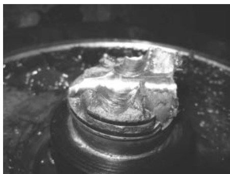
Figure 26.3 Example of failure involving stress concentration.
