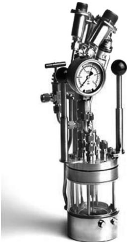
Figure 24.8 Chemical process analyzer. (Photograph courtesy of Fauske and Associates, LLC.)
