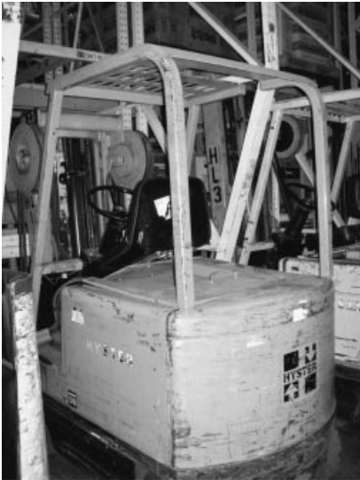
Figure 14.9 Overhead guard protection.
