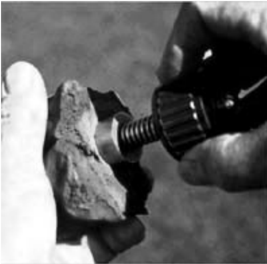
Figure 8.5 Shearvane application. (Courtesy OSHA.)
