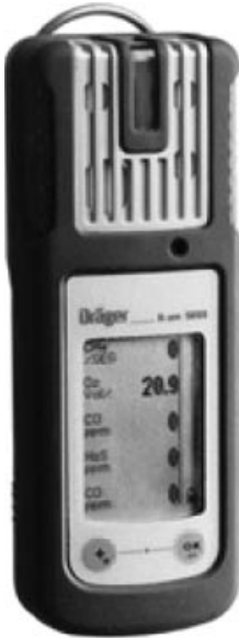
Figure 7.1 Multi-gas detector. A multi-gas detector can be used to monitor for explosive atmospheres. (Photograph courtesy of Safety, Inc.)
