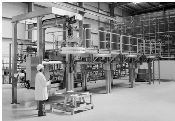
Figure 4.16. Picture of an installation of continuous separation by chromatography; this installation is used in the pharmaceutical industry to purify active ingredients, typically optical enantiomers. In the background, the installation for solvent recycling. Photo credit: NovaSep
