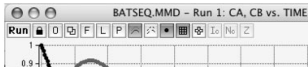
Fig. 2 The example BATSEQ has been run with the Colors, Data Points and Grid selected. From left: Lock, Overlay, Table, Legend, Parameters, Colors, Dashed Lines, Data Points, Grid, Value Output and Zoom.
