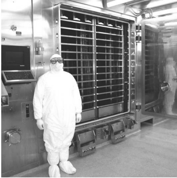
FIGURE 41.4 Image of typical commercial-scale freeze-dryer. This freeze-dryer has a total shelf surface area of 39 m 2 . It has 24 shelves and 6 trays per shelf. This image is obtained from Pfizer Kalamazoo manufacturing facility.
