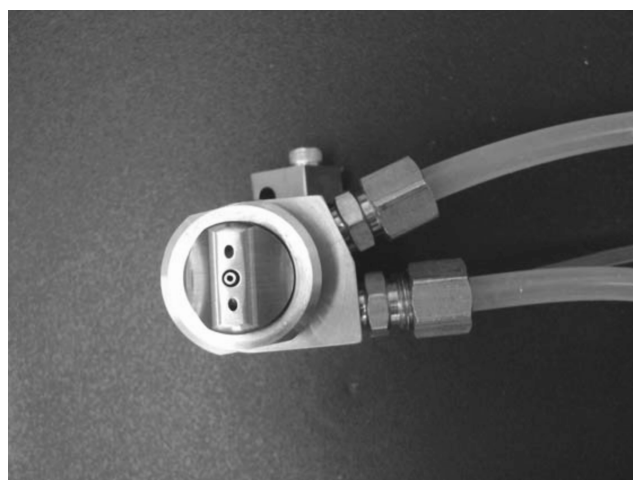
FIGURE 40.6 Front view of a laboratory-scale spray gun for tablet coating (Schlick fluid nozzle and air cap with spray gun body by Vector Inc.).
