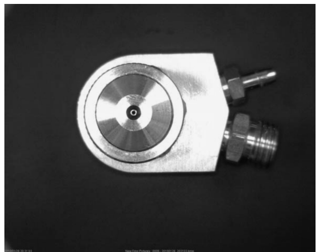
FIGURE 40.10 Front view of a laboratory-scale spray gun for tablet coating (Spraying Systems fluid nozzle and air cap with spray gun body by Vector Inc.).
