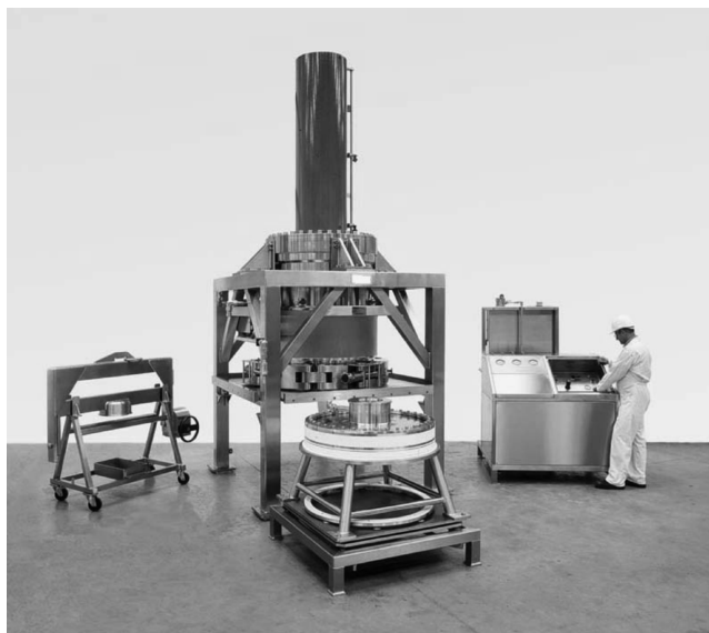
FIGURE 18.6 A 1 m internal diameter dynamic axial compression column for large scale high-performance liquid chromatography. The gray cylinder above the column is part of the hydraulic system to maintain pressure on the piston during packing an operation. Components of the piston assembly are seen in the foreground. Photograph courtesy of Novasep Inc.
