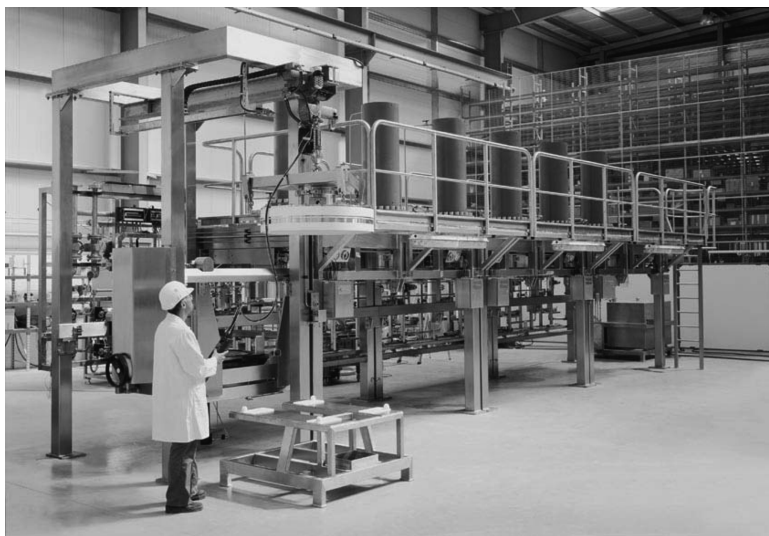
FIGURE 18.7 A six-column simulated moving bed unit. Each column has 1 m internal diameter. The unit was designed to operate in a Varicol process. Photograph courtesy of Novasep Inc.
