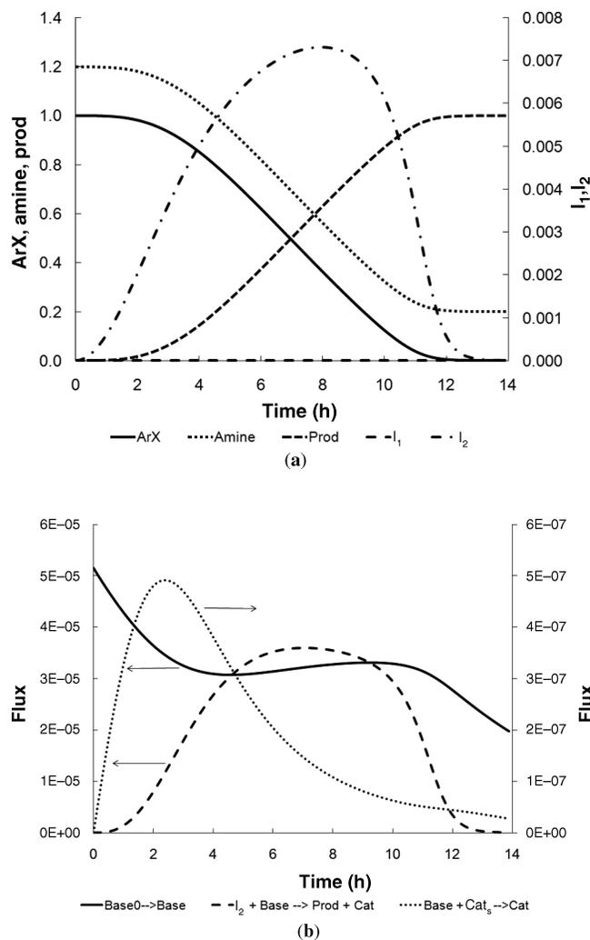
**FIGURE 10.6** Selected species and flux profiles for the synthesis mechanism shown in Figure 10.2. Part (a) shows the concentration profiles for species ArX, Amine, Prod,  $I_1$ , and  $I_2$ . Part (b) shows the flux profiles for reactions  $\text{Base}_0 \rightarrow \text{Base}$ ,  $I_2 + \text{Base} \rightarrow \text{Prod} + \text{Cat}$ , and  $\text{Base} + \text{Cat}_s \rightarrow \text{Cat}$ .
