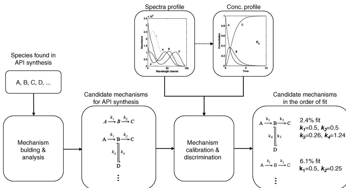
**FIGURE 10.1** Activities in API synthesis mechanism development including mechanism building, analysis, calibration, and discrimination. Both concentration and spectra profile data are used for mechanism calibration and discrimination.
