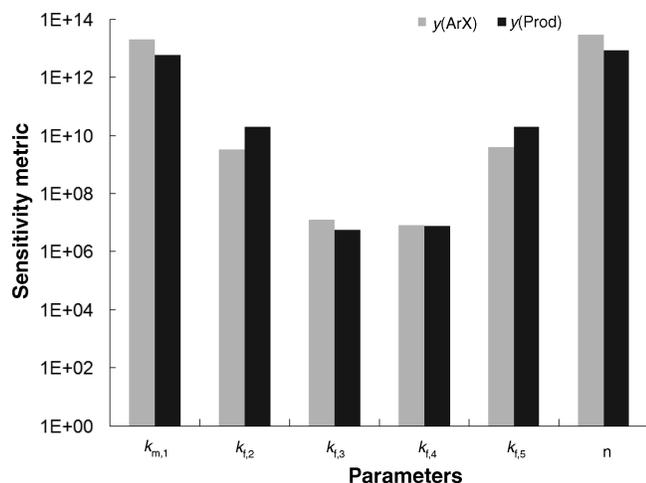
**FIGURE 10.10** Global sensitivity analysis results for the synthesis mechanism shown in Figure 10.2 for species ArX and Prod. The importance of the parameters, as measured by the averaged sensitivity metric, is valid not for a single set of parameter values but rather a four-order magnitude range of parameter values.
