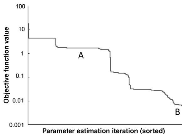
**FIGURE 10.12** Parameter estimation objective function versus multistart iteration number (sorted) for 46,656 samples. The flat, plateau regions correspond to locally optimal solutions that were found from several initial parameter values. Overlay plots corresponding to two parameter estimates, marked A and B, are shown in Figure 10.13.
