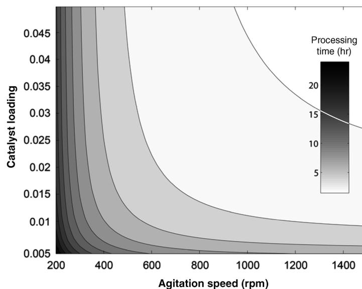
**FIGURE 10.16** Operating map for reactor operation for the synthesis described in Figure 10.2. The  $x$ -axis is the agitator speed and the  $y$ -axis is the catalyst loading. The contour plot shows the residence time in hours required to achieve the desired product yield. This figure indicates that operation is most sensitive to agitator speed at low rpm.
