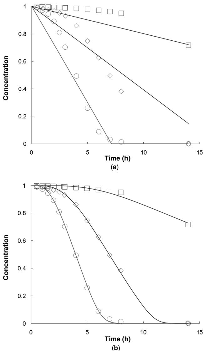
**FIGURE 10.13** Results of the OpenChem multistart parameter estimation for the mechanism shown in Figure 10.2. Part (a) shows the overlay plot for a locally optimal, but poor fit. Part (b) shows the overlay plot for the best parameter fit obtained and is clearly superior to the other fit.
