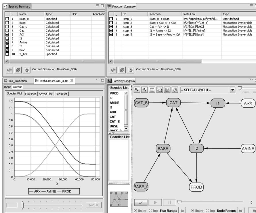
**FIGURE 10.5** OpenChem interactive four-panel Simulation Explorer. The upper left and upper right panels contain a summary of the species and reactions, respectively. The lower left and lower right panels contain the Plotting Environment and Pathway Diagram, respectively. These panels interact, providing a convenient overview of the mechanism behavior.
