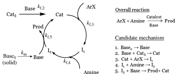
**FIGURE 10.2** Example API synthesis mechanism. Overall, an aryl halide reacts with an amine in the presence of a catalyst and strong base to form the desired aryl amine product. The schematic on the left shows the proposed mechanism steps, including formation of intermediate species. The corresponding candidate synthesis mechanism is shown on the right.
