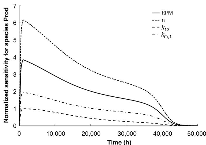
**FIGURE 10.8** Normalized parametric sensitivities for species Prod with respect to several parameters.
