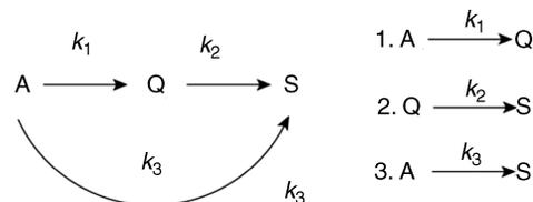
**FIGURE 10.14** Schematic of a synthesis mechanism involving three species and three reactions. Reactant A is converted to main product, S, directly and through an intermediate species Q.
