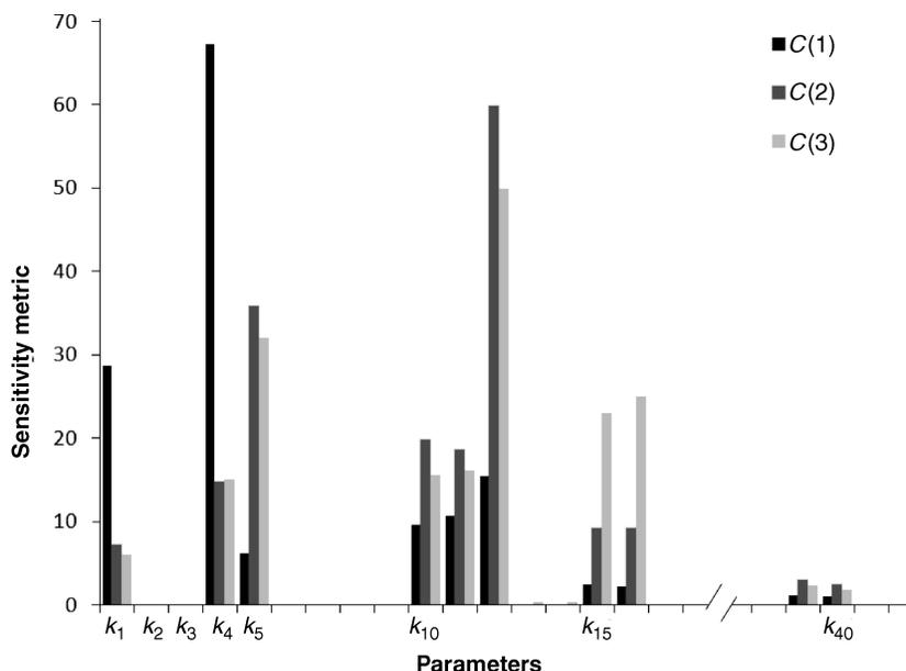
**FIGURE 10.11** Global sensitivity analysis results for a reaction mechanism involving 30 species and 42 parameters with results shown for three key model outputs,  $C(1)$ ,  $C(2)$ , and  $C(3)$ . The importance of the parameters, as measured by the averaged sensitivity metric, is valid not for a single set of parameter values but rather a four-order magnitude range of parameter values.
