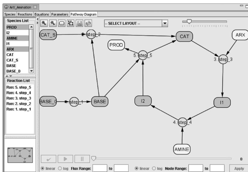
**FIGURE 10.4** OpenChem form for specifying a mechanism in graphical format. Species are denoted by round-cornered rectangles and reactions are denoted by circles. Arrows point from the reactant nodes to the reaction nodes and from the reaction nodes to the product nodes. A list of species and reactions is shown on the left of the form. Selecting one or more species and/or reactions in these lists will highlight the corresponding nodes in the graph.
