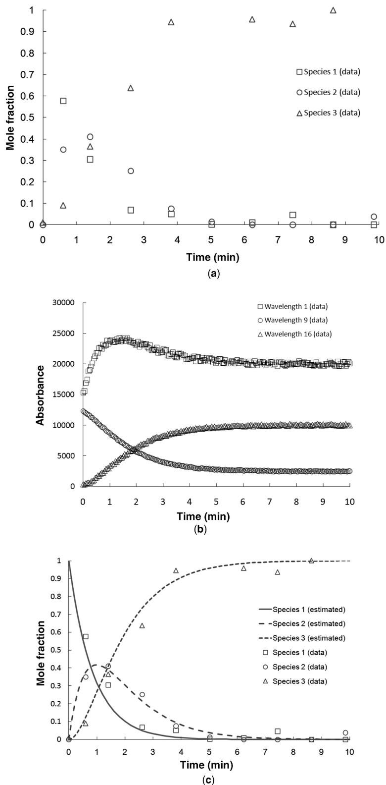
**FIGURE 10.15** Input data and results for the mixed data calibration method implemented in OpenChem. Part (a) shows the measured concentration data (algorithm input). Part (b) shows the measured spectra data (algorithm input). Part (c) shows the overlay plot for the optimal solution (simulated profiles and measured concentration data).
