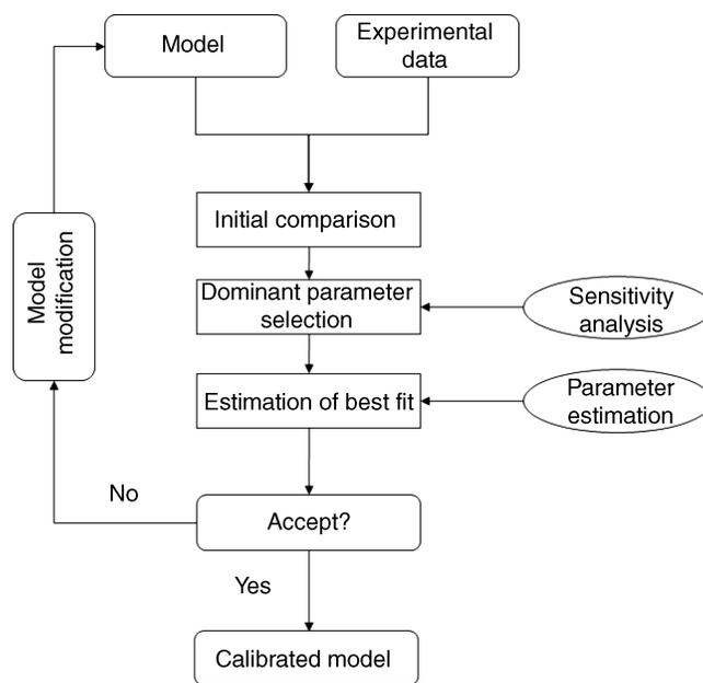
**FIGURE 10.9** Calibration workflow. The major steps involved in model calibration are illustrated in this figure. Techniques that can be applied are shown in the ellipses. An important part of this workflow is model modification; deficiencies in the model and/or data are often uncovered during model calibration.
