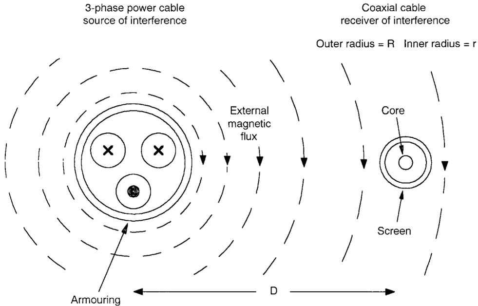
**Figure 13.13** Mutual coupling between spaced out cables.
