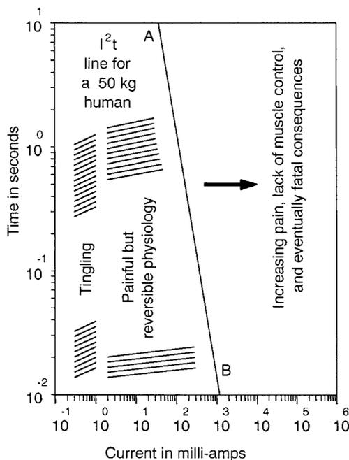
**Figure 13.1** Intensity of electric shock for human beings.
