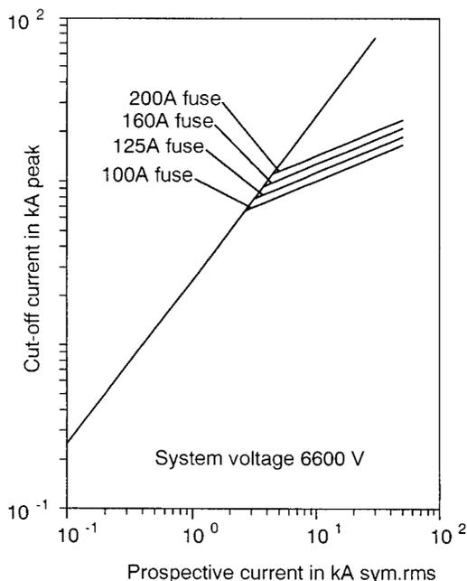
**Figure 8.3** Peak cut-off current versus prospective symmetrical rms current for typical fuses in the range of 100 A to 200 A.
