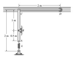
$$T_1 + V_1 = T_2 + V_2$$
