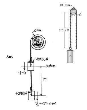
**18–43.** Solve Prob. 18–42 if the chain has a mass per unit length of 0.8 kg/m. For the calculation neglect the portion of the chain that wraps over the sprocket.
