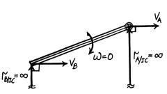
\*18–32. The assembly consists of two 15-lb slender rods and a 20-lb disk. If the spring is unstretched when  $\theta=45^{\circ}$  and the assembly is released from rest at this position, determine the angular velocity of rod AB at the instant  $\theta=0^{\circ}$ . The disk rolls without slipping.
