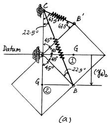
•18–53. A spring having a stiffness of  $k=300 \, \text{N/m}$  is attached to the end of the 15-kg rod, and it is unstretched when  $\theta=0^{\circ}$ . If the rod is released from rest when  $\theta=0^{\circ}$ , determine its angular velocity at the instant  $\theta=30^{\circ}$ . The motion is in the vertical plane.
