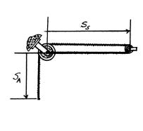
**18–62.** The motion of the uniform 80-lb garage door is guided at its ends by the track. If it is released from rest at  $\theta=0^\circ$ , determine the door's angular velocity at the instant  $\theta=30^\circ$ . The spring is originally stretched 1 ft when the door is held open,  $\theta=0^\circ$ . Assume the door can be treated as a thin plate, and there is a spring and pulley system on each of the two sides of the door.
