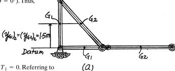
**Kinetic Energy:** Since the panel is at rest in the closed position,  $T_1 = 0$ . Referring to Fig. b, the IC for BC is located at infinity. Thus,
