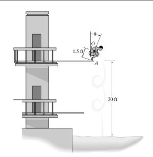
During the fall no forces act on the man to cause an angular acceleration, so  $\alpha = 0$ .
