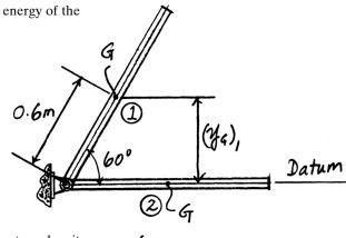
**Kinetic Energy.** Since the rod is at rest at position (1) and is required to stop when it is at position (2),  $T_1 = T_2 = 0$ .
