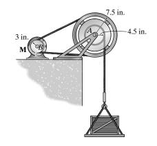
**18–19.** The wheel and the attached reel have a combined weight of 50 lb and a radius of gyration about their center of  $k_A = 6$  in. If pulley B that is attached to the motor is subjected to a torque of M = 50 lb·ft, determine the velocity of the 200-lb crate after the pulley has turned 5 revolutions. Neglect the mass of the pulley.
