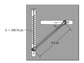
**Potential Energy:** With reference to the datum in Fig. a, the gravitational potential energy of the rod at positions (1) and (2) is
