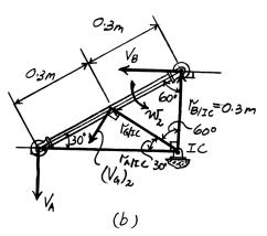
**18–54.** If the 6-kg rod is released from rest at  $\theta = 30^{\circ}$ , determine the angular velocity of the rod at the instant  $\theta = 0^{\circ}$ . The attached spring has a stiffness of k = 600 N/m, with an unstretched length of 300 mm.
