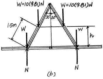
**18–22.** Determine the angular velocity of the two 10-kg rods when  $\theta = 90^{\circ}$  if they are released from rest in the position  $\theta = 60^{\circ}$ . Neglect friction.
