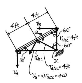
**18–63.** The 500-g rod AB rests along the smooth inner surface of a hemispherical bowl. If the rod is released from rest from the position shown, determine its angular velocity at the instant it swings downward and becomes horizontal.
