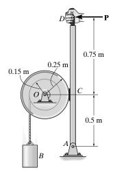
\*18–8. The drum has a mass of 50 kg and a radius of gyration about the pin at O of  $k_O=0.23$  m. If the 15-kg block is moving downward at 3 m/s, and a force of P=100 N is applied to the brake arm, determine how far the block descends from the instant the brake is applied until it stops. Neglect the thickness of the handle. The coefficient of kinetic friction at the brake pad is  $\mu_k=0.5$ .
