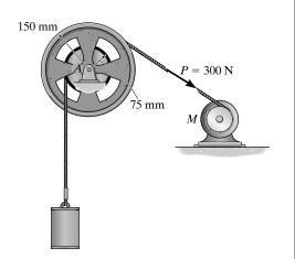
**Kinetic Energy and Work:** Since the reel rotates about a fixed axis,  $v_C = \omega_r r_C$  or  $\omega_r = \frac{v_C}{r_C} = \frac{v_C}{0.075} = 13.33 v_C$ . The mass moment of inertia of the reel about its mass centers is  $I_A = m_r k_A^2 = 25 (0.125^2) = 0.390625 \text{ kg} \cdot \text{m}^2$ . Thus, the kinetic energy of the system is
