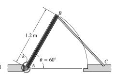
**Potential Energy:** With reference to the datum in Fig. a, the gravitational potential energy of the panel at positions (1) and (2) is
