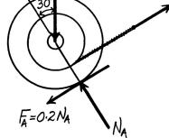
**18–14.** The spool has a weight of 500 lb and a radius of gyration of  $k_G = 1.75$  ft. A horizontal force of P = 15 lb is applied to the cable wrapped around its inner core. If the spool is originally at rest, determine its angular velocity after the mass center G has moved 6 ft to the left. The spool rolls without slipping. Neglect the mass of the cable.
