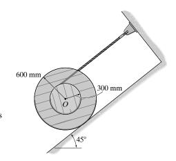
**18–26.** The spool has a mass of 100 kg and a radius of gyration of 400 mm about its center of mass O. If it is released from rest, determine its angular velocity after its center O has moved down the plane a distance of 2 m. The coefficient of kinetic friction between the spool and the inclined plane is  $\mu_k = 0.15$ .
