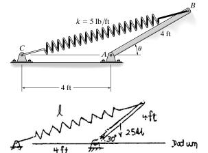
•18–65. The 25-lb slender rod AB is attached to spring BC which has an unstretched length of 4 ft. If the rod is released from rest when  $\theta = 30^{\circ}$ , determine the angular velocity of the rod the instant the spring becomes unstretched.
