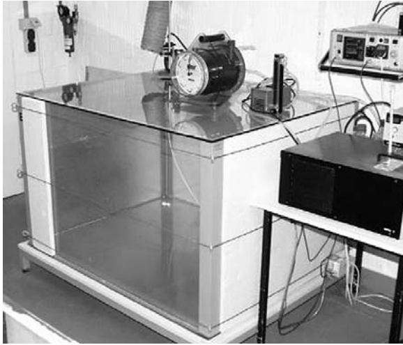
Fig. 2 View of a 1-m 3 emission test chamber used in WKI (Photo: T. Salthammer)
