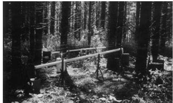
Figure 2.11 Throughfall troughs sitting beneath a pine tree canopy. This collects rain falling through the canopy over the area of the trough. It is sloping so that water flows to a collection point.
