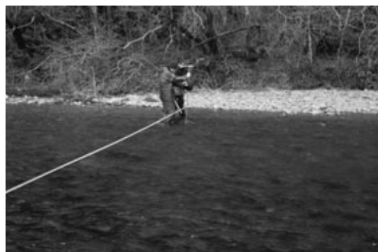
Figure 5.7 Flow gauging a small stream.
