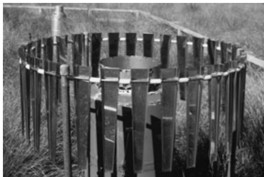
Figure 2.8 Baffles surrounding a rain gauge to lessen the impact of wind turbulence. The gauge is above ground because of snow cover during the winter.
