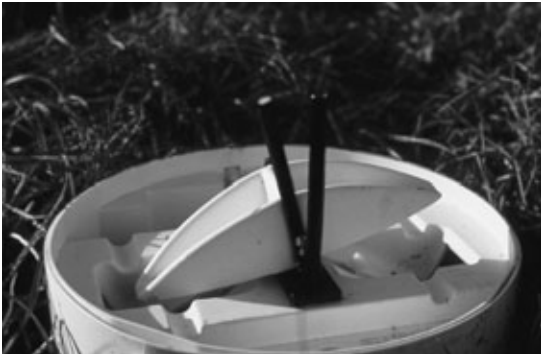
Figure 2.10 The insides of a tipping-bucket rain gauge. The 'buckets' are the small white, triangular reservoirs. These are balanced and when full they tip over bringing the black arm past the other stationary arm. In doing so a small electrical current is passed to a data logger.
