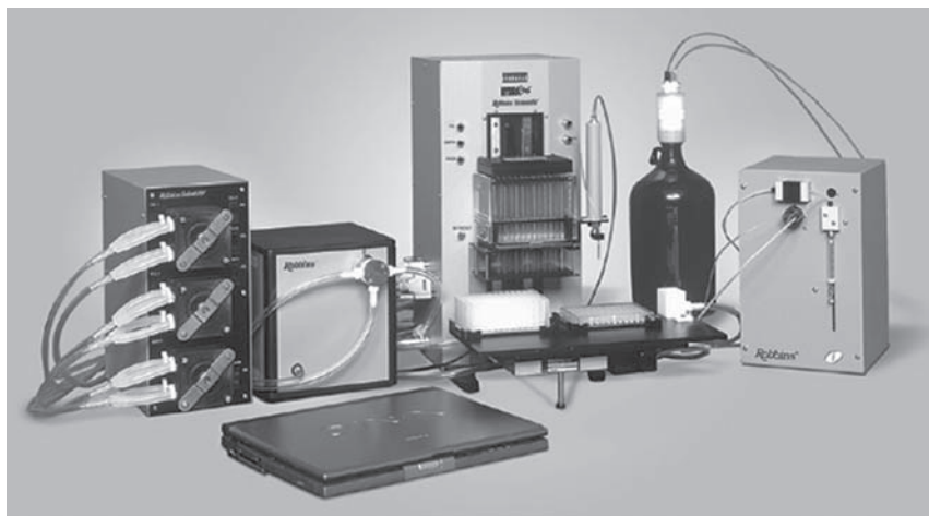
Fig. 3. The Hydra-Plus-One System. The NanoFill has a dispensing nozzle (internal diameter of 125\ \mu\text{M} ) connected to a 25-in-long tube. The sample is aspirated from a 0.6 mL microtube into the nozzle and is separated from the system fluid ( \text{H}_2\text{O} ) by an air gap of 0.75\text{--}1\ \mu\text{L} . Therefore, as is the case with the syringes, the sample does not dry or evaporate once inside the noncontact dispenser.
