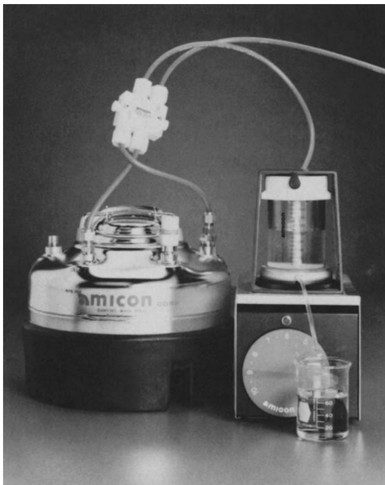
Fig 3. Stirred UF cell on magnetic stirrer. The reservoir and selector valve are used for desalting or buffer exchange.
