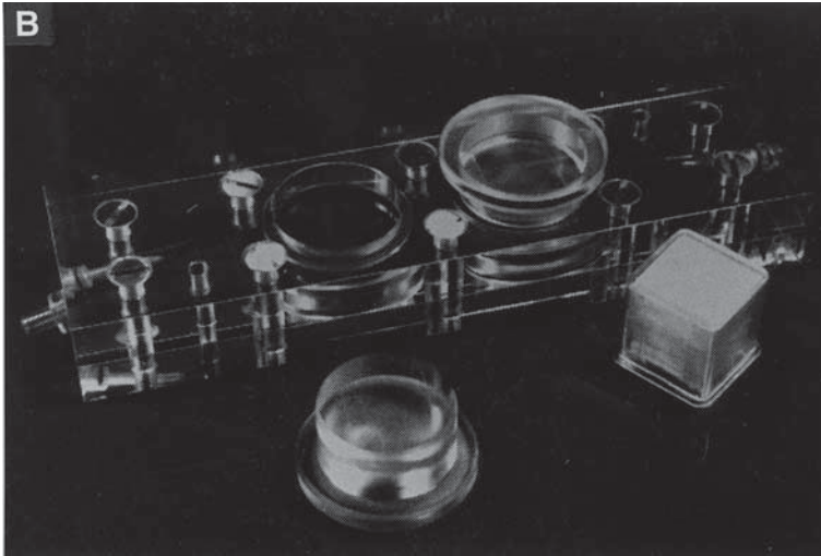
Fig. 1B. Picture of the perfusion chamber. The coverslip is mounted on the plug, introduced in the chamber, and exposed to flow.
