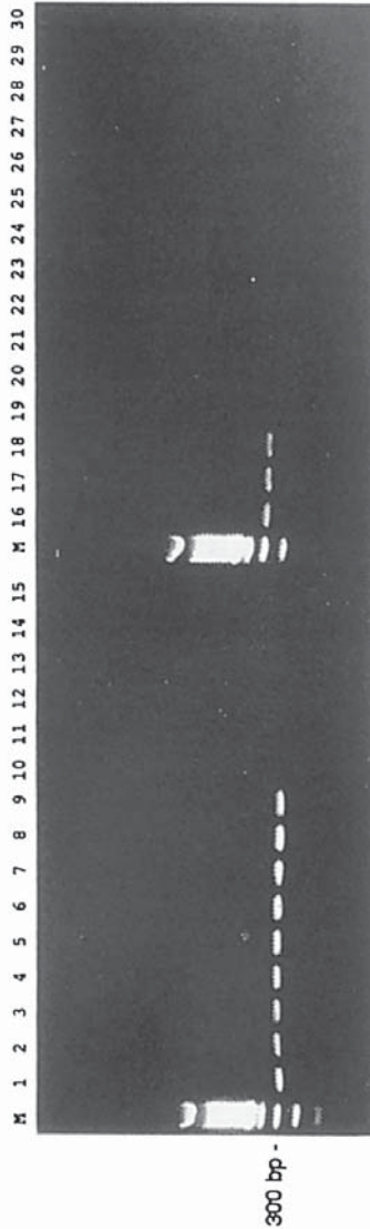
Fig. 1. Identification of V. cholerae using PCR based on the 16S–23S rRNA intergenic spacer region. Lanes M, molecular weight marker (100 bp ladder): 1, V. cholerae O1 classical ATCC 14035 T ; 2–5, V. cholerae O1 El Tor clinical isolates; 6–9, V. cholerae O139 clinical isolates; 10, V. mimicus ATCC 33653 T ; 11–15, V. mimicus isolates; 16–18, V. cholerae non-O1/non-O139 isolates; 19, V. aestuarianus ATCC35048 T ; 20, V. alginolyticus ATCC17749 T ; 21, V. campbellii ATCC25920 T ; 22, V. carchariae ATCC35084 T ; 23, V. diazotrophicus ATCC33466 T ; 24, V. fischeri ATCC7744 T ; 25, V. fluvialis ATCC33809 T ; 26, V. furnissii ATCC35016 T ; 27, V. hollisae ATCC33564 T ; 28, V. natriegens ATCC14048 T ; 29, V. salmonicida ATCC43839 T ; 30, V. vulnificus ATCC27562 T . T Type strain.
