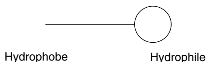
FIGURE 7.10 ► Schematic of a surfactant molecule.
