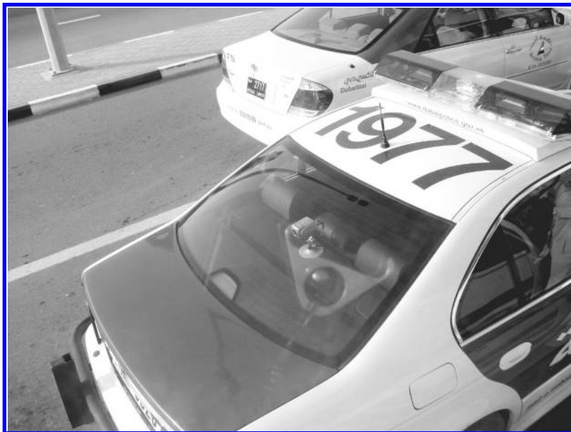
Photo 7-1. Patrol car in Dubai. Note the camera fixed in the rear of the vehicle. This camera is controlled from police headquarters and not from the vehicle. It also transmits to police headquarters. An officer at headquarters may observe the actions of both the officer and the surroundings by viewing the camera.
